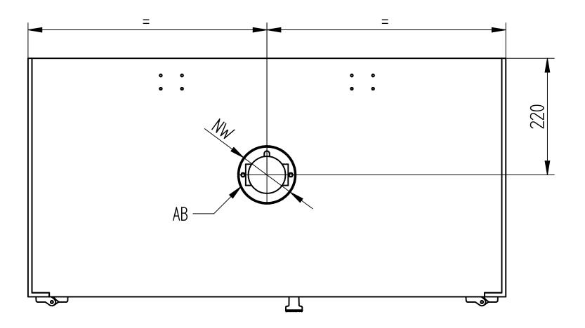
NW: 110, with adapter 75 AB: Exhaust air connection
